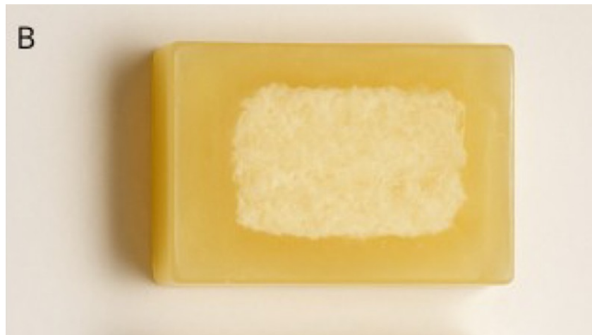
Figure B: Yellowish due to temperature above 65°C. The higher the temperature, the greater the intensity of the yellowish color, indicating quality deviation in sample processing and embedding.
