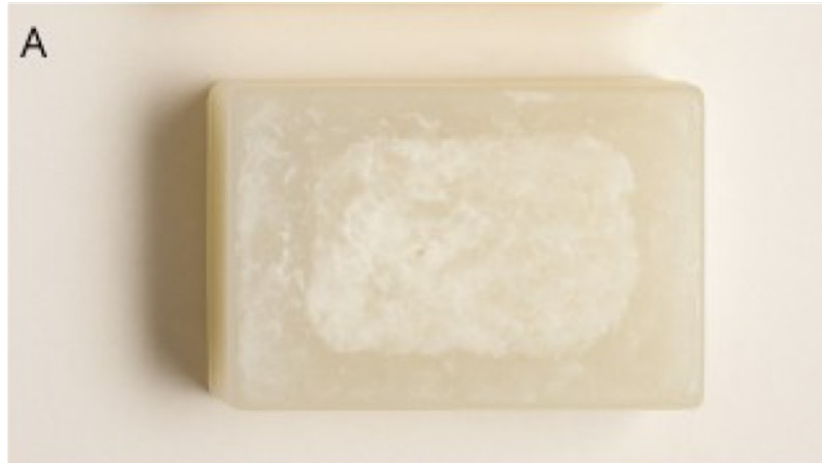
Figure A: At temperatures up to 65°C, the paraffin coloration does not change, ensuring sample preservation.
